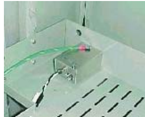
Figure 3-11; Location of SPI in Equipment Tray
